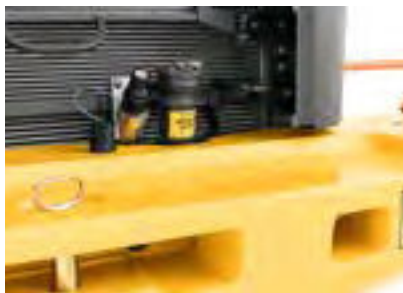
Fast fill fueling system
