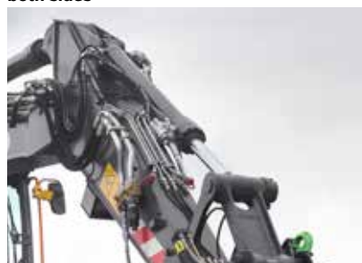
Load holding valves on bucket cylinders, both sides
