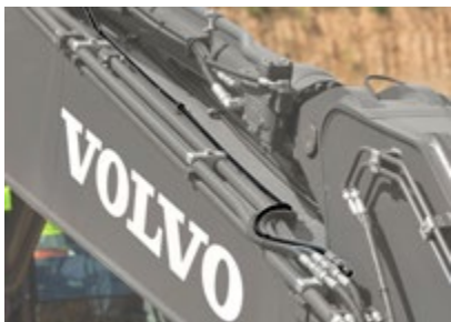
Oil drain line
