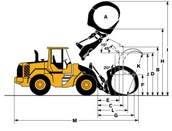
L60F Sales code: WLA82194 Operating weight (incl. logging cw 120 kg): 12 210 kg Operating load: 3450 kg
