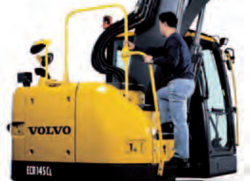
• 3-point, multi-purpose access with hand rail for ease and safety.
