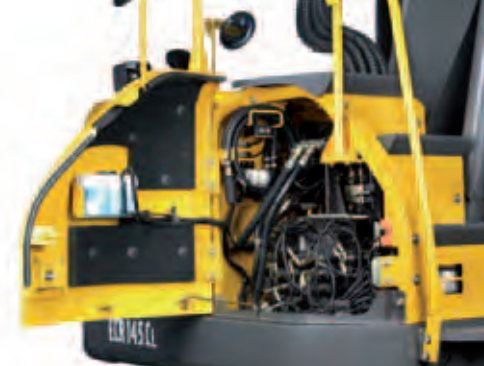
• Wide open, ground level service area provides easy hydraulic valve access.
