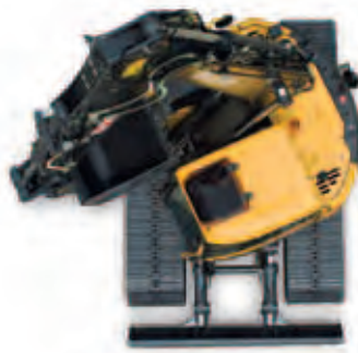
• Rounded design with a compact swing radius.
