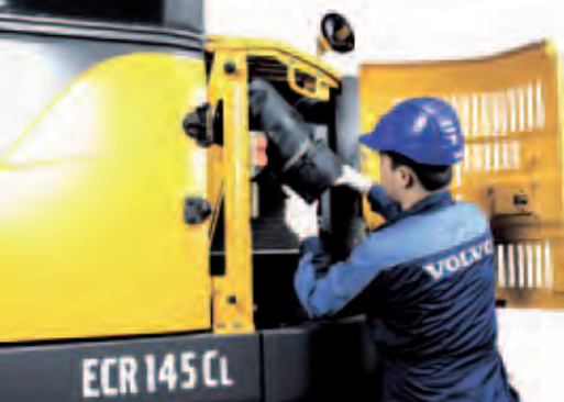
• Ground level air filter access.
